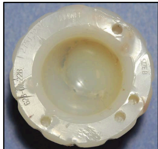
Figure 2: Stereomicrograph of a Sequentially Annealed acetabular liner that was implanted for 5.0 years.
