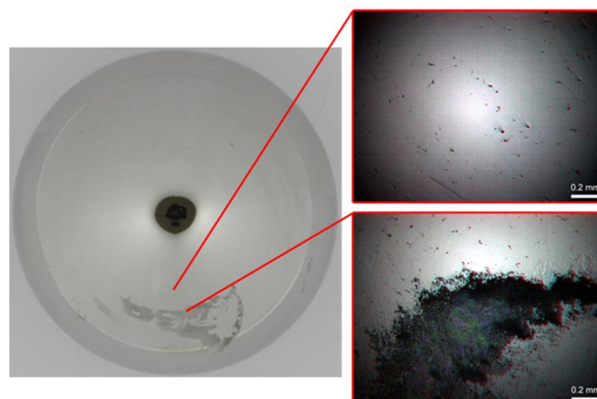
Figure 5: Representative femoral head of group 2 after 3 million cycles. The anterior position is orientated to the right side of the picture.
