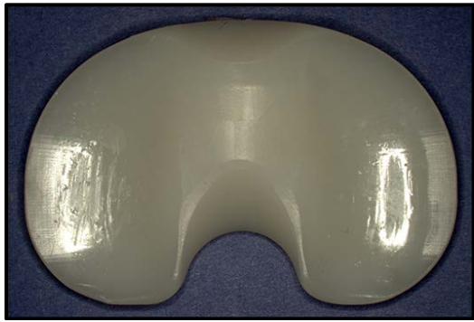
Figure 3: Stereomicrograph of a Sequentially Annealed tibial insert that was implanted for 5.5 years. Note the burnishing, scratching, and impressions from 3 rd body wear.
