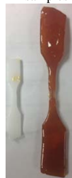
Figure 2: A tensile specimen of control PE (left) and Vitamin E infused PE (right)
