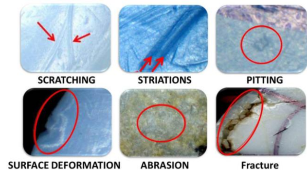
Fig. 3. Primary damage modes observed on UHMWPE glenoids.
