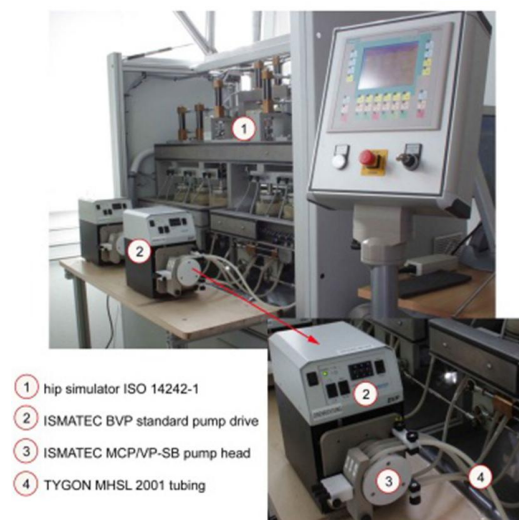
Figure 1: EndoLab® six station hip joint simulator according to ISO 14242-1 modified with two peristaltic pumps.
